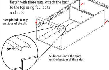
**7.** Next, attach the sill (Ref. No. 6) to the sides, as shown above. Place nuts loosely on each of the studs and slide the ends of the sill into the slots on both sides of the unit. Then, securely tighten the nuts.
