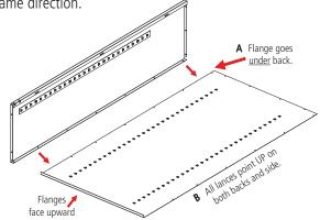
**4.** Attach the right side (Ref. No. 3) to the back in the same manner as you did in step 3, again, making sure that the flange is around the back and that the lances on the shelf adjustment strips are pointed in the same direction as those on the back and left side.
